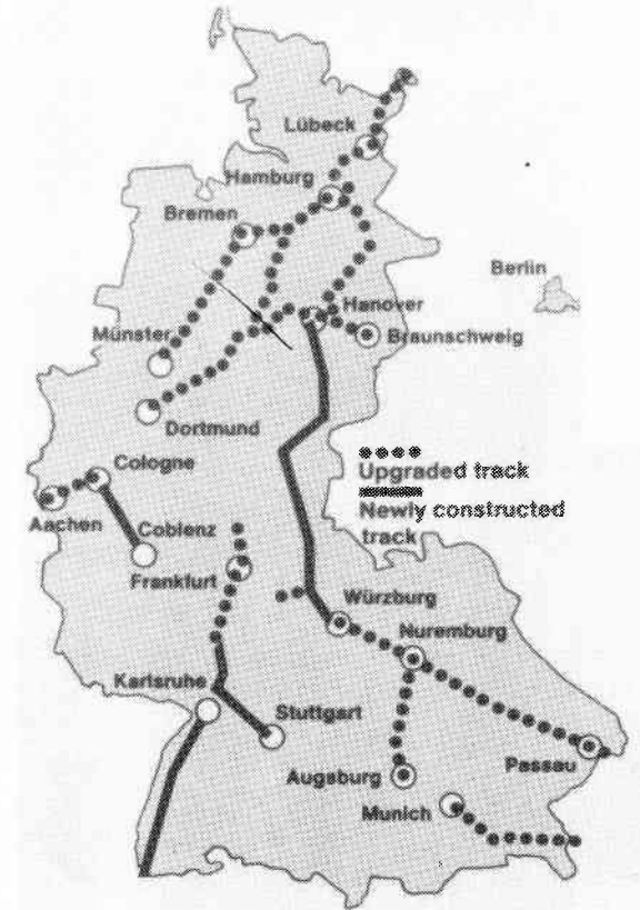
Sixty-two tunnels have to be built for the new Hanover—Würzburg rail link. This much-frequented route is the centre-piece of a programme to modernize and expand the German railway network. Thirteen stretches of track are to be upgraded and four rebuilt altogether.
